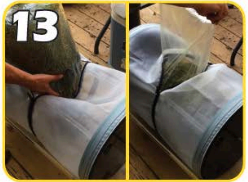
Load Material by unzipping secondary/loading zipper to open position. Place entire bag into drum cylinder and carefully empty contents into drum while removing bag. *or use hand scoop to load material
