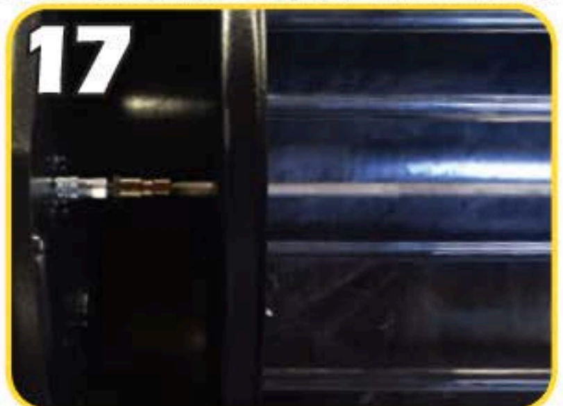
Gently place rotary/quick release side of drum shaft into receiving groove.
